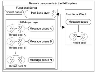
Figure 6. Architecture of network communication components.
