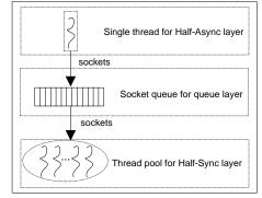
Figure 4. Half-Sync/Half-Async architectural pattern[10].
