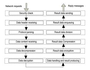
Figure 7. A complex network data handling flow.
