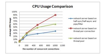
Figure 14. CPU Usage comparison.
