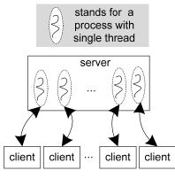
Figure 2. process-per-connection model.
