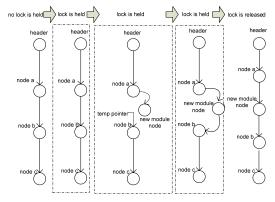
Figure 9. add a new module into data handling flow.
