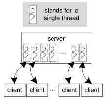
Figure 1. thread-per-connection model.
