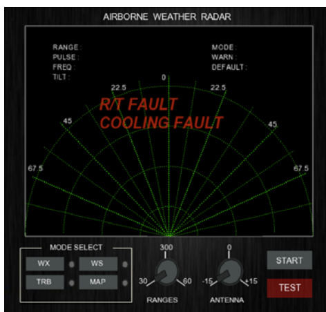
Figure 11. Self-testing fault indication
