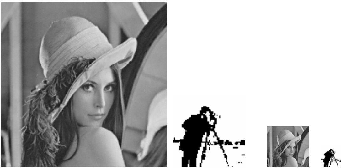
Figure 7. Enlarged watermarked image and extracted watermark (ratio is 3) Reduced watermarked image and extracted watermark (ratio is 0.4).
