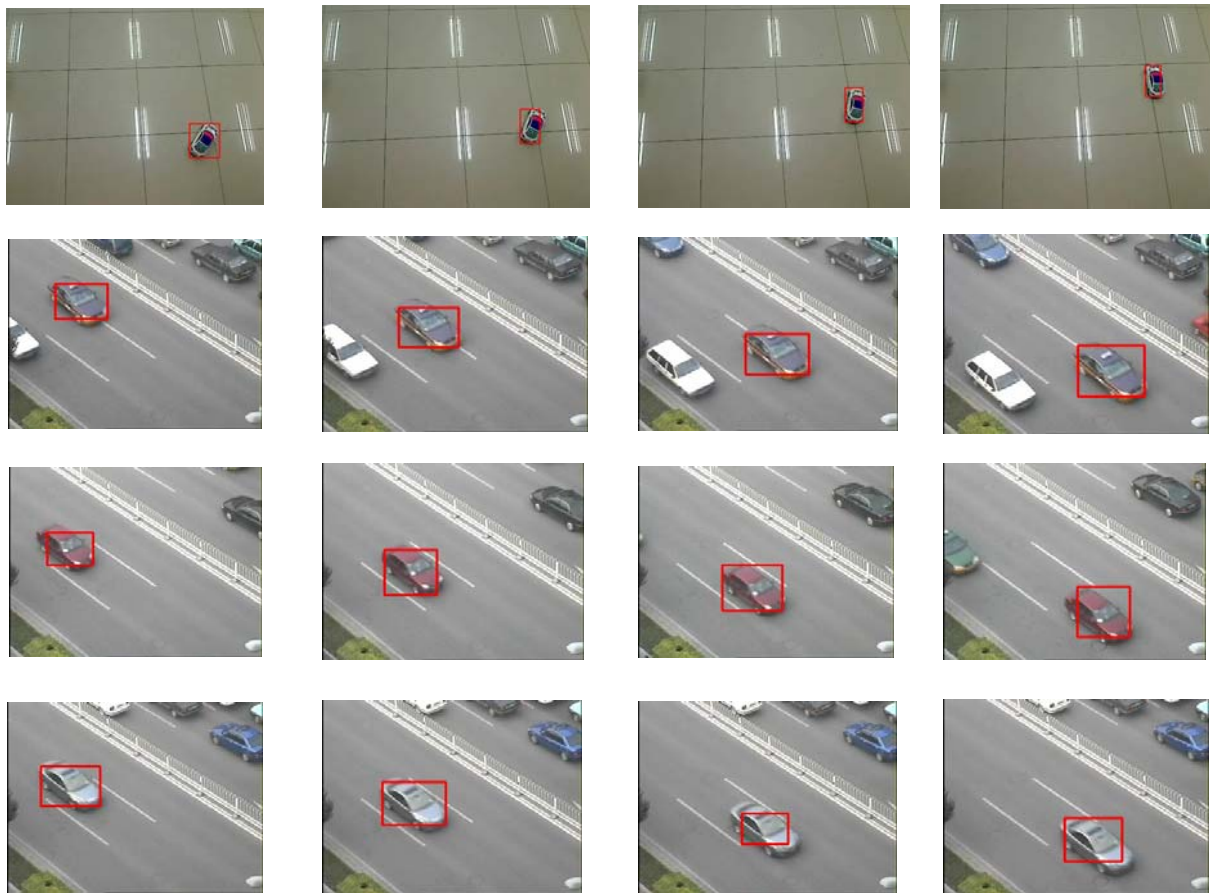
Fig. 6 The images of single target tracking result using the proposed algorithm in AI car and traffic video.
