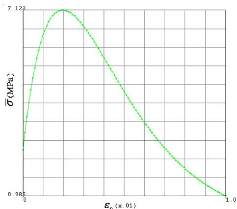
Figure 4. The equivalent stress-equivalent plastic strain relationship of mortar
