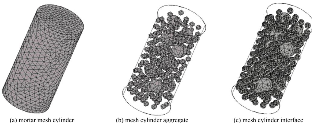
Figure3. The mesh dissection of three dimensional random aggregate (sphere aggregate)
