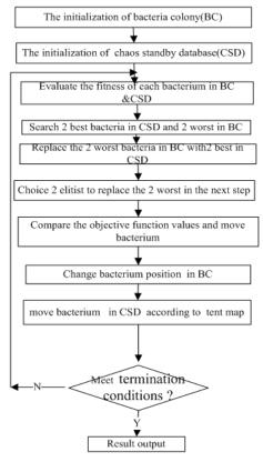
Figure 2. Flow chart of novel CHBCC algorithm
