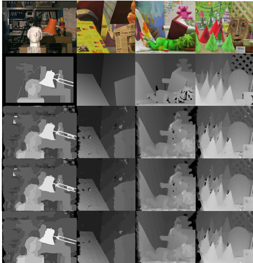
Figure 1. Disparity maps for the “Tsukuba”, “Venus”, “Teddy” and “Cones” images. The top is the reference images. The second row is the truth disparity maps. The third row is the results using L1 norm function. The fourth row is the results using the TAD cost function. The last row is our optimal results using the CA_OWF method.
