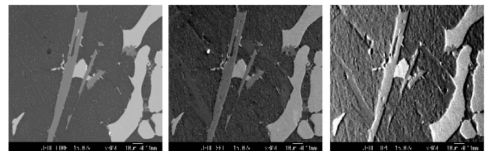
Figure 2: BSE 、 SEI and TOPO image of same sample(has been registered)
