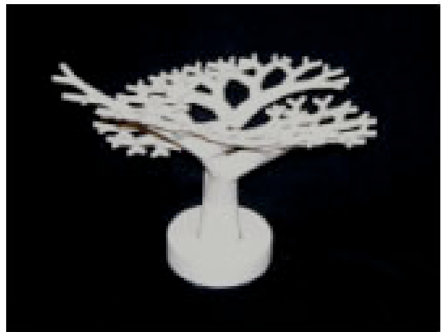
Figure 4. A plaster model of a tree, originally designed on the computer screen and then output to a 3D printer. [1]
