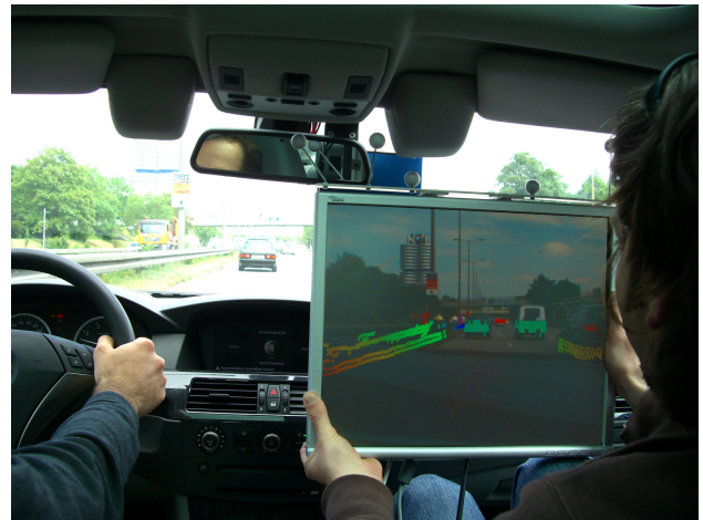
(a) One can see the laser-scanner data superimposed on the vehicles and the guardrail
