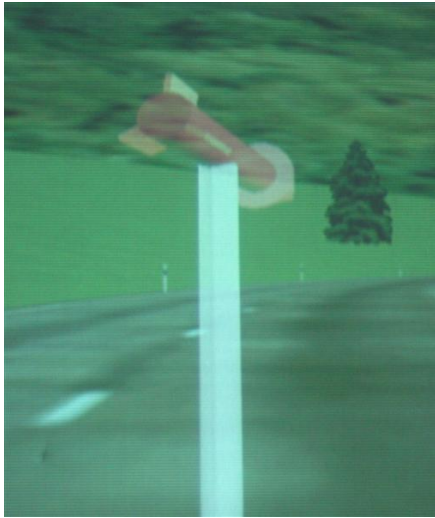
Figure 14. An indicator for the direction of an imminent danger in the car's environment, shown in the Head-up Display
