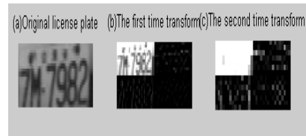
Fig. 19. Rain day 7M-7982 license plate HDWT two times transform.
