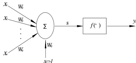
Figure1. The unit of processing
