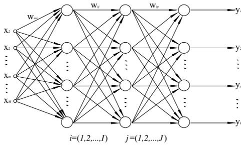
Figure 2. The model of BP net
