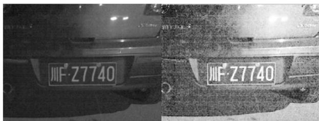
Fig.5 (a) L component of license plate with complicated background scene. (b) enhanced L component of license plate nighttime environment scene using our method.
