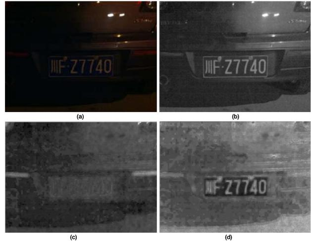
Fig.4 Conversion RGB to La\*b\* color space (a) original image, (b) L component, (c) colored a\* component, (d) colored b\* component.
