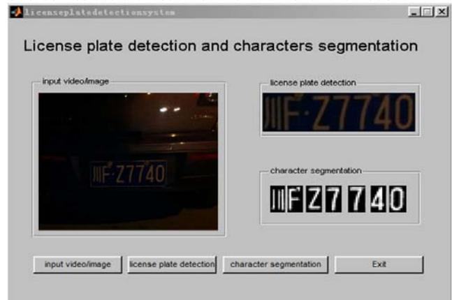
Fig.9 the nighttime license plate detection and segmentation system developed based on our proposed method.
