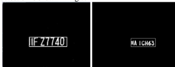
Fig.7 The results of license plate detection using the proposed method.
