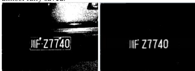
Fig.6 (a) the original binary image after vertical edge extraction. (b) the result of long curve and random noise removing from the original binary image.
