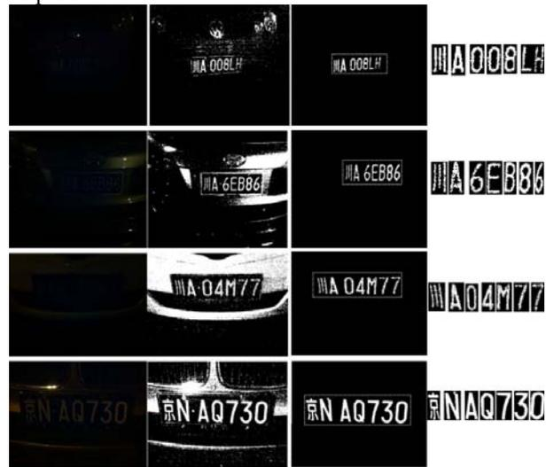
Fig.10 the first column is original nighttime license plate image with complicated background scene, the second column is experimental results using Sobel operation, the third column is experimental results of license plates detection, the fourth column is experimental results of character segmentation of license plates.
