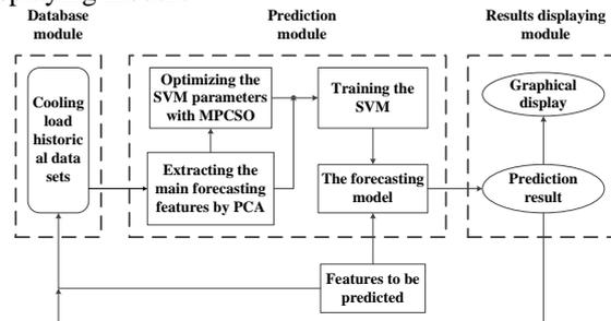
Figure 8. The structure of the MPCSO-SVM based short-term cooling load forecasting model.
