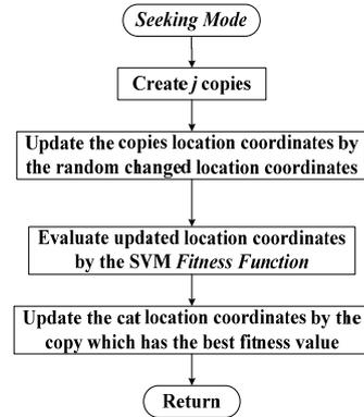
Figure 2. The flow chart of seeking mode in MPCSO-SVM.
