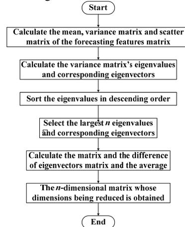
Figure 7. The flow chart of extracting the main forecasting features by PCA.
