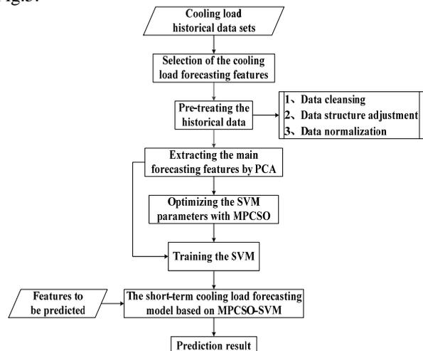
Figure 5. The short-term cooling load forecasting model flow chart.
