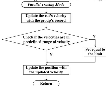
Figure 3. The flow chart of Parallel tracing mode in MPCSO-SVM.
