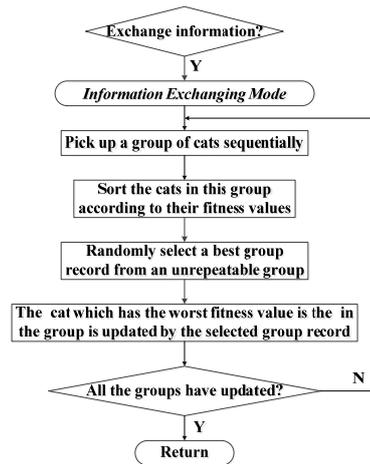
Figure 4. The flow chart of the information exchanging mode in MPCSO-SVM.
