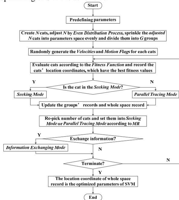
Figure 1. The flow chart of prediction parameters optimization with MPCSO-SVM.
