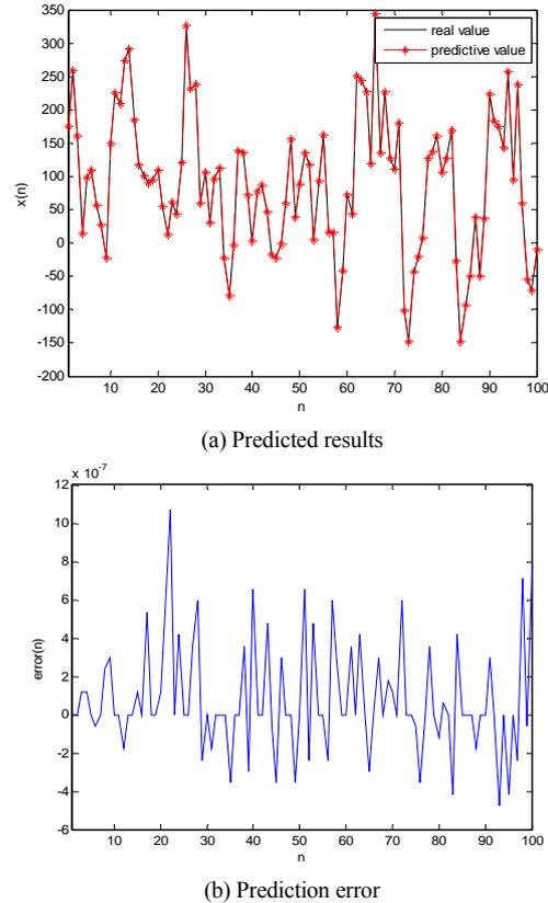
Figure 3. Prediction of the first category of underwater acoustic signal by RBF neural network
