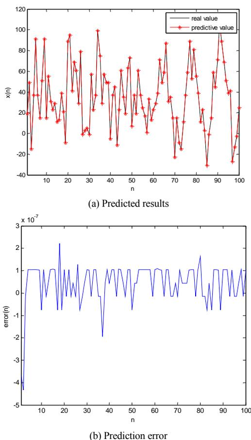
Figure 5. Prediction of the third category of underwater acoustic signal by RBF neural network
