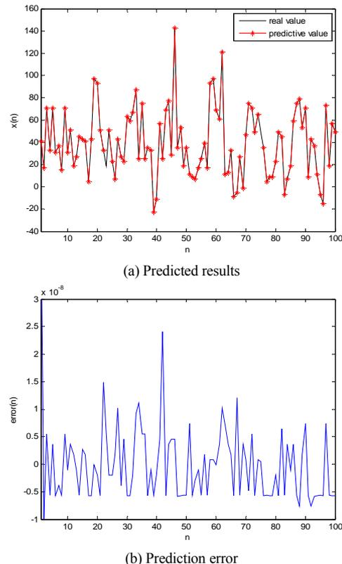
Figure 4. Prediction of the second category of underwater acoustic signal by RBF neural network
