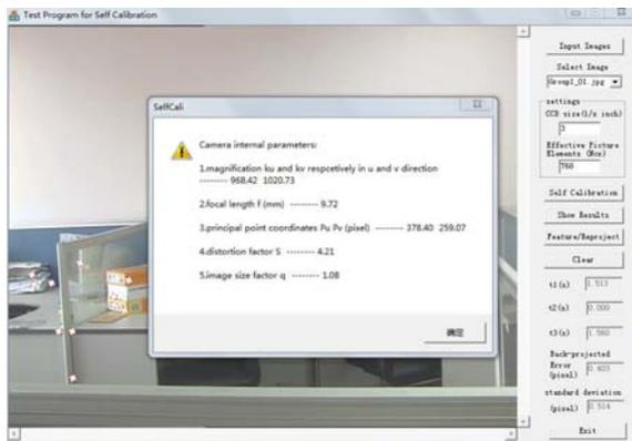
Figure 6. Display the self-calibration results of camera in a popped dialog
