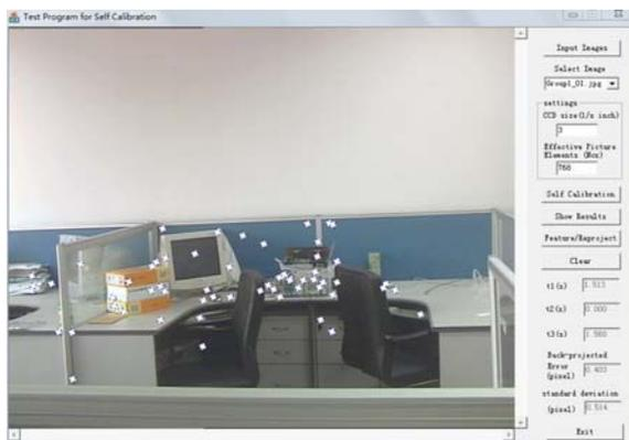
Figure 7. Show the back-projected 2D feature point
