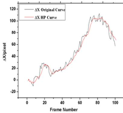
Figure 7. Measured curve and filtered result for vector  $\Delta X$
