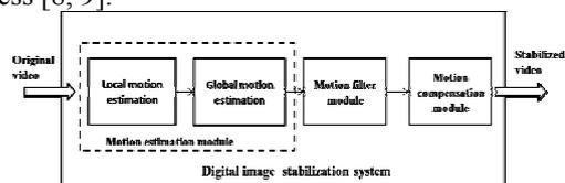
Figure 1. Flow diagram of DIS system
