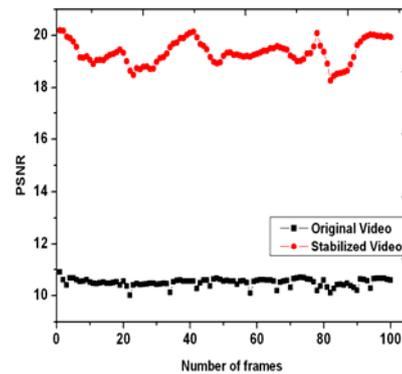
Figure 10. The PSNR curve of the original video and stabilized video
