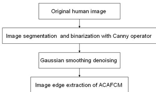
Figure 2. Flowchart of image processing
