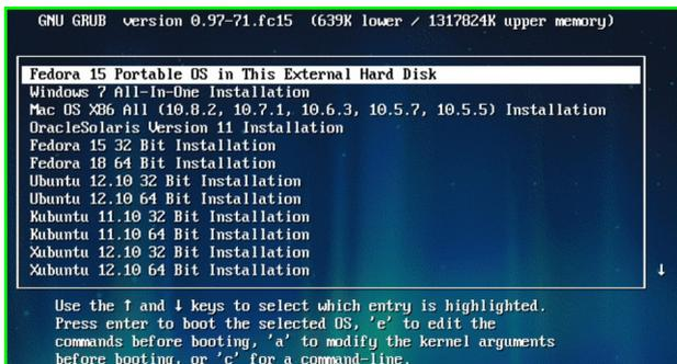
Figure 6. Displayed boot menu on booting a PC with this usb HD
