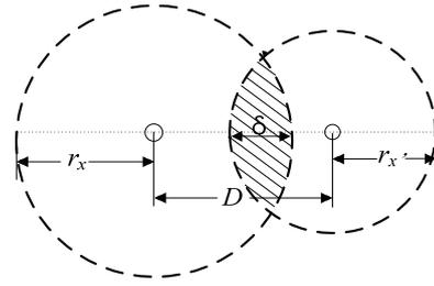
Figure 1. the overlap between two detectors.
