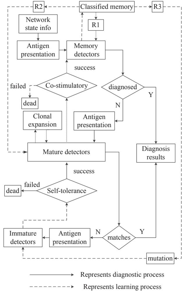
Figure 2. Network Fault Diagnosis Model.
