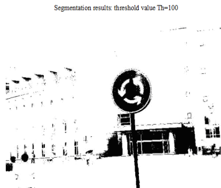
Figure 3. Segmentation effect diagram of the traffic sign image based on iterative threshold
