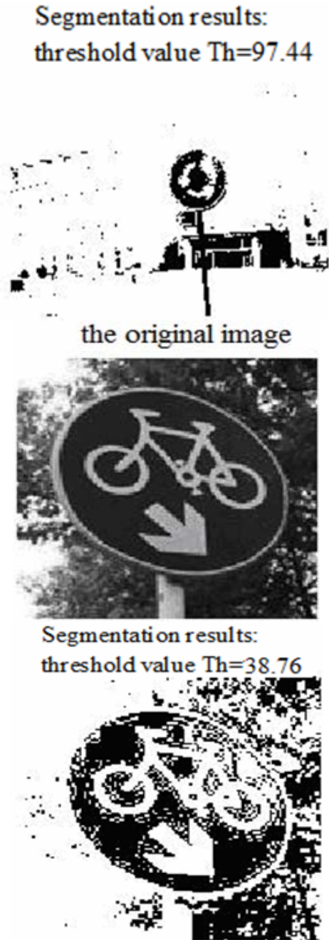
Figure 2. Effect drawings of traffic signs segmentation based on Ostu algorithm.
