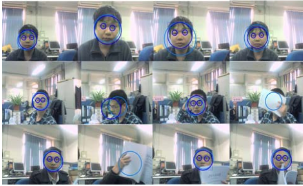
Figure8. Recognition test in the case of the, multi-scale variations, the driver head movement and pose variation.
