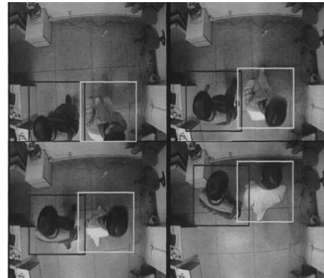
Figure 2. Multi-target Tracking with Interference Region
