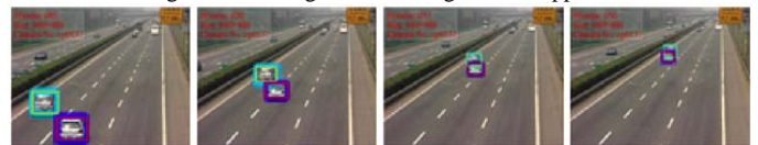
Figure 4. Color-similar vehicles track when partial occlusion occurs
