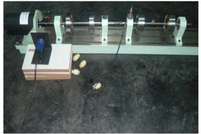
Figure 3. Rotor vibration simulation test-bed
