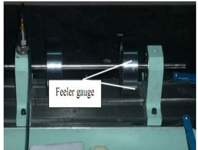
Figure 4. Adjustment of the feeler gauges thickness for misalignment fault
