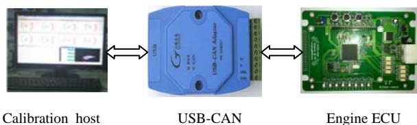
Figure 9. Calibration bench for engine ECU
