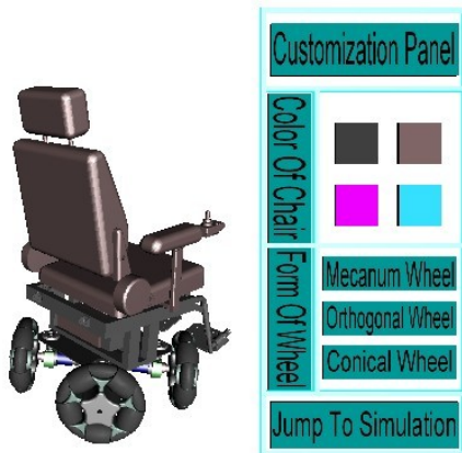
(b) Wheelchair with orthogonal wheel
