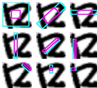
Figure 11. Some haar-like features used in the cascade classifier of radical “kou”
