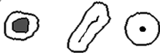
a. polygon based buffer b. polyline based buffer c. point based buffer
