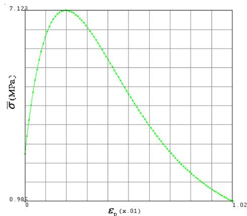
Figure 4. The equivalent stress-equivalent plastic strain relationship of mortar
