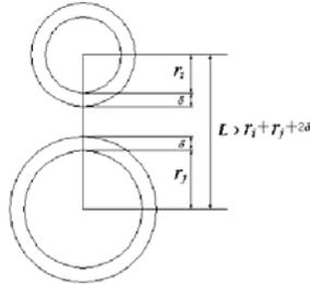
Figure 1. The shortest distance between the aggregates
