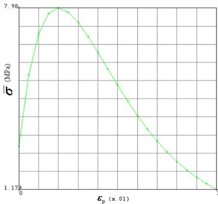
Figure 6. The equivalent stress-equivalent plastic strain relationship of RA
