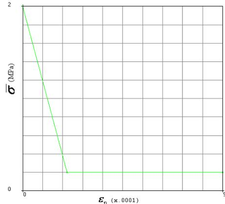
Figure 7. The equivalent stress-equivalent plastic strain relationship of natural aggregate interface
