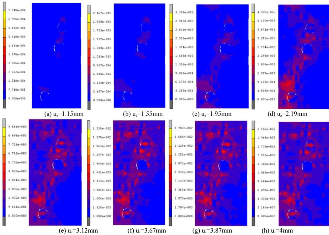
Figure 11. The variation picture of the cracking strain distribution of the middle longitudinal section
