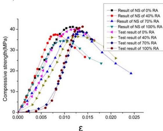
Figure 13. The compress stress-strain relationship curve for recycle concrete cylinder specimen
