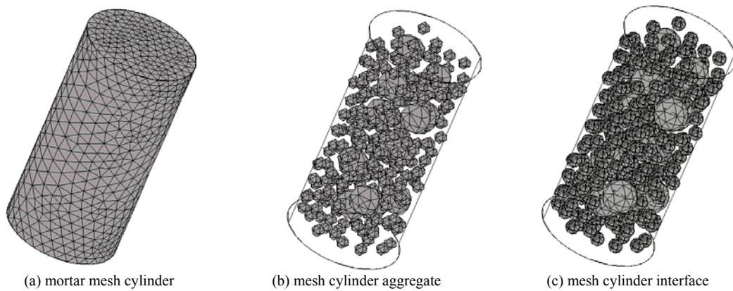
Figure3. The mesh dissection of three dimensional random aggregate (sphere aggregate)
