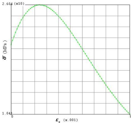
Figure 5. The equivalent stress-equivalent plastic strain relationship of natural aggregate
