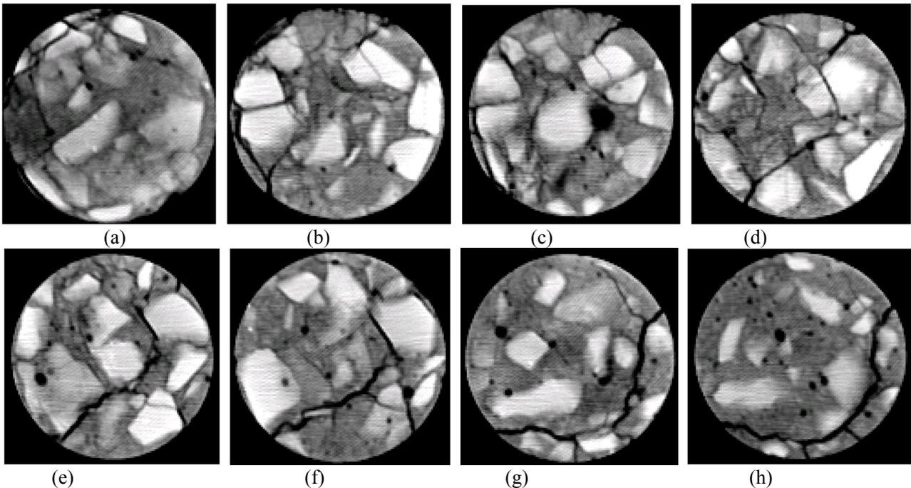
Figure 12. The cross-section damage pictures of cylinder specimen
