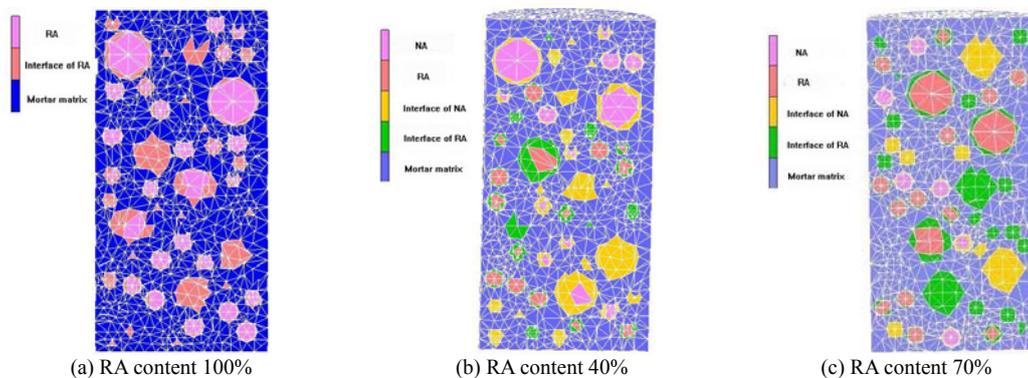
Figure 9. The material information of RC cylinder specimen
