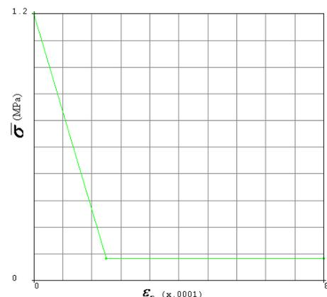
Figure 8. The equivalent stress-equivalent plastic strain relationship of RA interface
