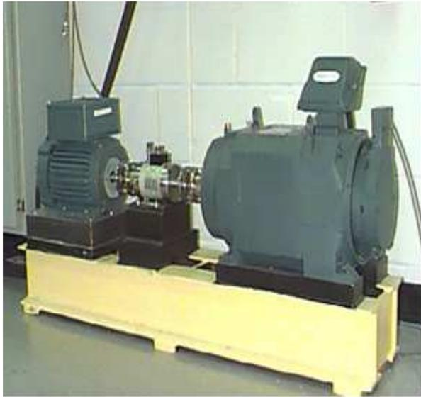
Figure 1. Rolling bearing test experiment stand
