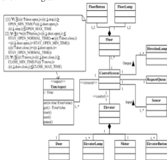
Figure 8. The Elevator Control System Class Diagram
