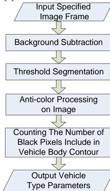
Figure5. Processing Flow of Vehicle Digital Image
