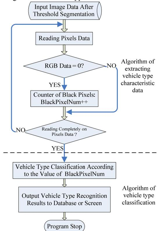
Figure11. Algorithm of Vehicle Type Recognition
