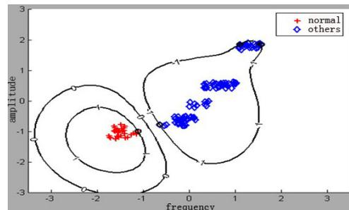
Figure.11 SVM1-normal and fault classification
