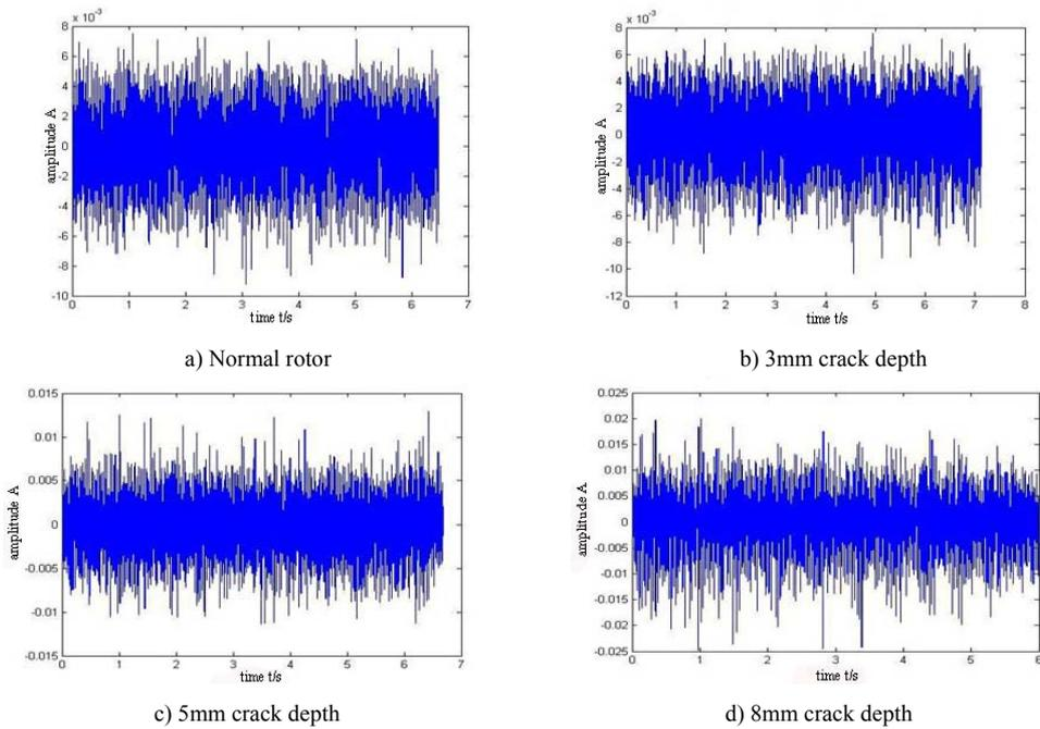
Figure.4 Time domain map of vibration signal at 1800r/min
