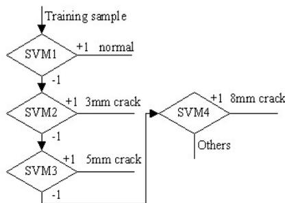
Figure.10 Multi-fault classifier of support vector machine
