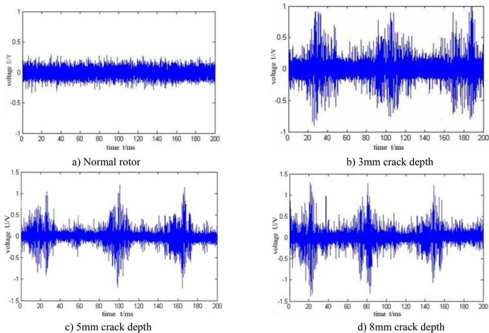
Figure.5 Time domain diagrams of acoustic emission signal at 1800r/min
