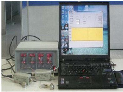
Figure.3 Acquisition system of AE signal.
