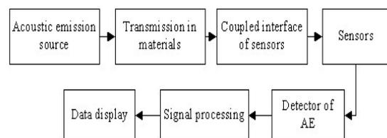
Figure.2 Schematic of acoustic emission testing.
