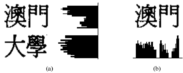
Figure 4. Character segmentation based on projection analysis. (a) Text separated by horizontal projection; (b) characters (and components) separated by vertical projection.
