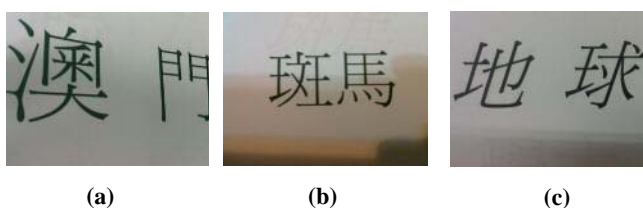
Figure 5. The captured images failure at recognition and translation - (a) shooting with perspective angle, (b) uneven lighting with shadow, and (c) text with italic font style.
