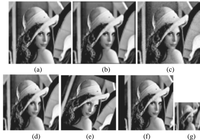
Fig.4. Invariant centroids which are marked as cross: (a)original image;(b) 3 \times 3 average filtered;(c) 5% Gaussian noise added;(d) JPEG compressed image with compression ratio of 70;(e) 20^\circ clockwise rotation of image plus cropping;(f) 30 pixels translated along x-axis;(g) scaled based on scaling factor of 0.5.
