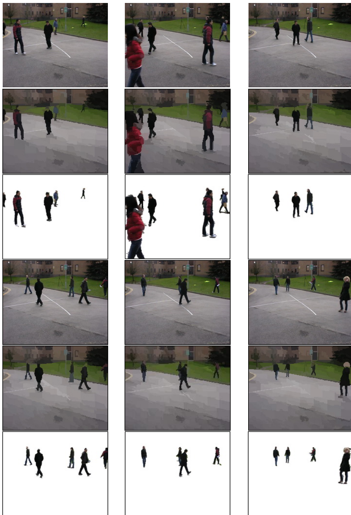
Figure 11. experimental results of PETS2009. First and forth row: input frame 678, 702,717,753,766,791; second and fifth row: segmentation results; third row and sixth row: segmentation result by the proposed method
