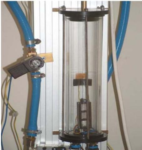
Figure 6. The remote experiment for phenomenological thermodynamics. A piston (top) runs in a glass cylinder compressing air. The temperature of the gas can be adjusted by a heater (bottom) and the pressure and the position of the piston are measured.
