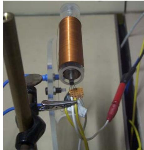
Figure 4. Setup of the remote experiment on hysteresis, the magnetic coil in the middle, Hall probe in front
