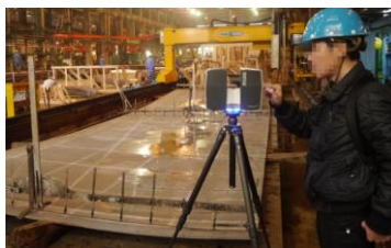
Fig.1. 3D laser scanner field data acquisition.
