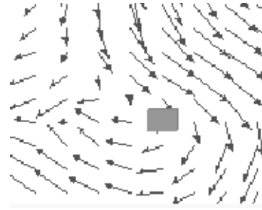
Figure 2. A typical example of a hard case for automatic detection: a strong local extremum of curl that triggers classical methods but does not match with a retentive structure. This map detail is taken from the surroundings of South Brittany.
